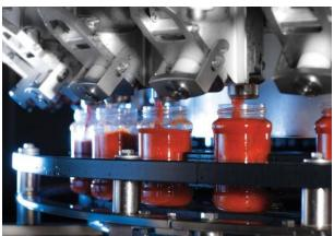
the sequence of the sauces packaged—for example, starting with plain tomato-based and moving to those with more ingredients—Barilla is able to reduce the frequency of total sanitization of the line. In this way, Sacchelli says the plant can produce up to five different recipes per week.
