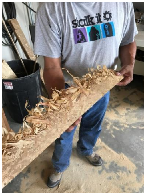
Figure 3: Trimmed edge from board highlighting the density obtained during the pressing process (Cornboard)
