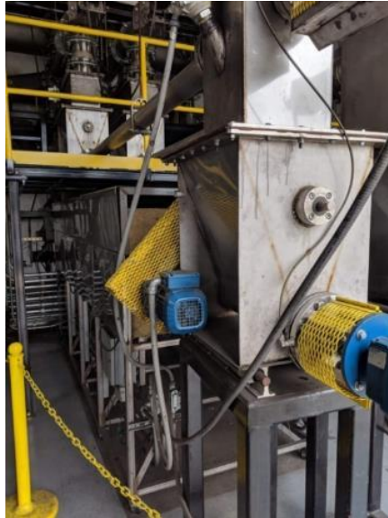
Figure 6: End view of feed housing to reactor body. Note the faint V-outline on flat plate, the moving feed floor prevents bridging blockages when handling bulkier biomass (Wampler's Farm Sausages)
