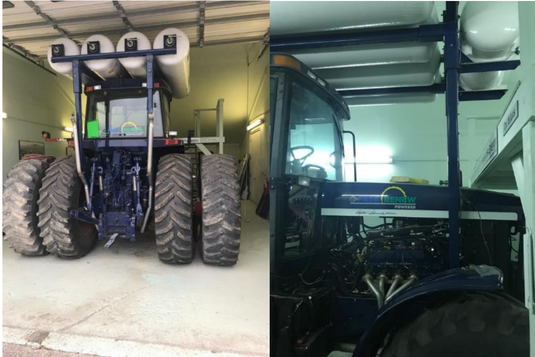
Figure 13: Hydrogen converted tractor at the Schmuecker family farm in Iowa. Note the hydrogen tanks mounted longitudinally above the cab as well as the smaller ammonia tank mounted cross ways at the front
