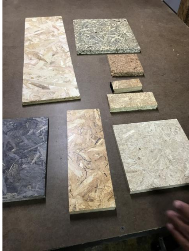
Figure 4: Trials of different plant fibres, resins, pressures and temperatures (Cornboard)
