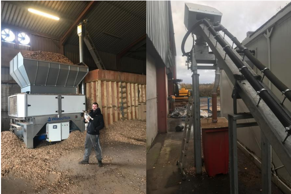
Figure 8: L: Tom Lifely showing wood chip dryer and screen; R: external to the shed showing the material feed augers entering and exiting the container modules
